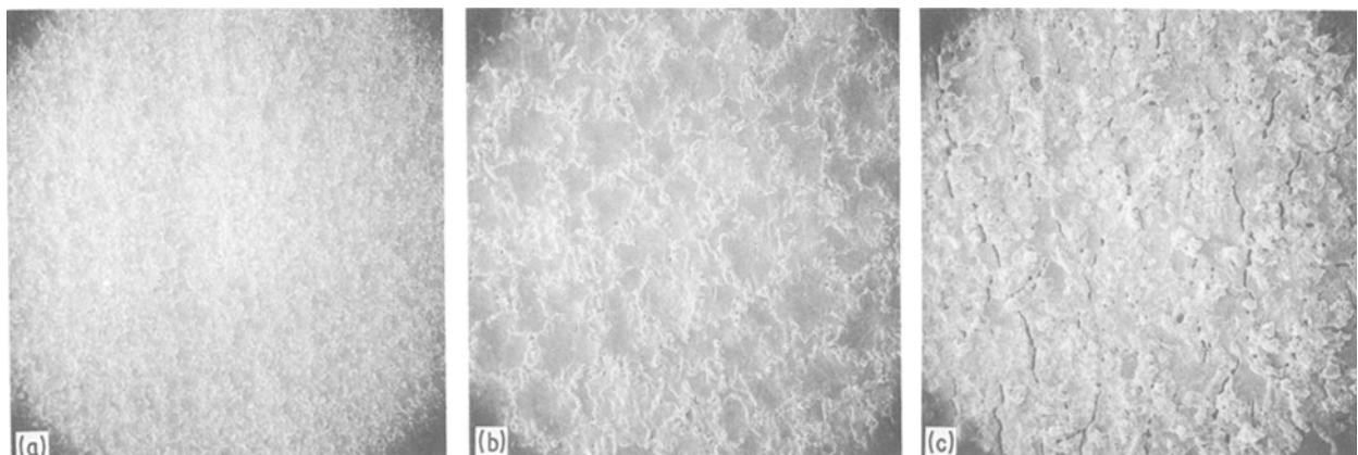
Figure 8 As Fig. 7 for 25% SiCw/Al EDM surface. (a) Fine, (b) medium, (c) coarse.
